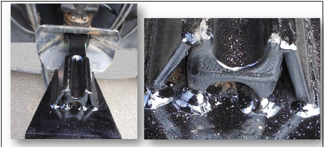
Figure 13: Example of poor installation: The gusset provides additional support but the lower edge of the drawbar eye is not fully welded to the drawbar. Furthermore, maintenance personnel are unable to check the lower-edge welds for cracking.
