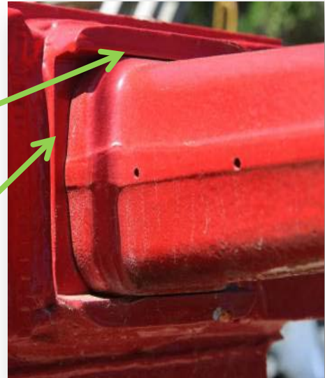
Figure 7: A drawbar eye with no visible wear or movement. Undisturbed paint around the drawbar eye indicates that there is no movement of the eye in the mounting block.
