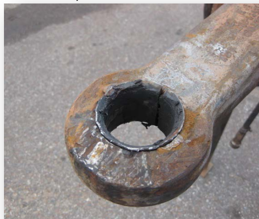
Figure 11: Heavily worn and damaged drawbar eye bush.
