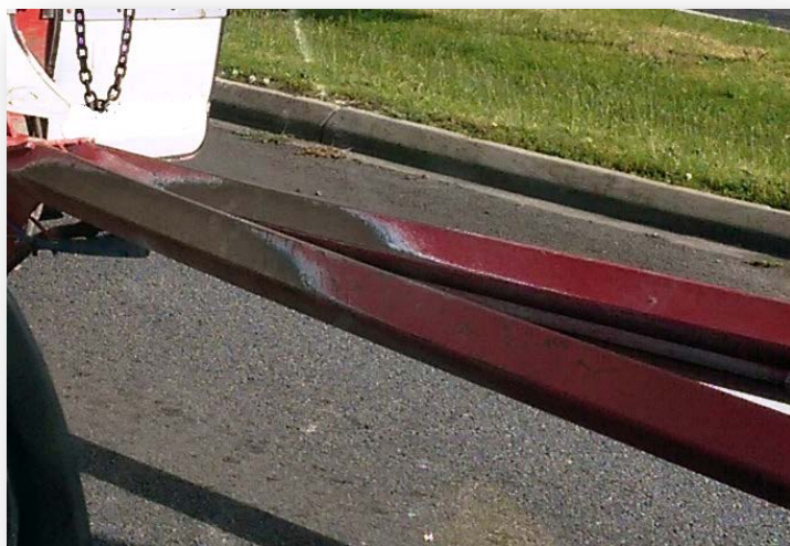
Figure 15: Wear on drawbar
